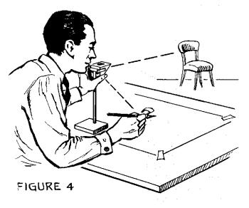
A practical hint to follow when using the "Mirror Lucida" is to use plenty of light on the drawing paper, and to have a well-lighted object as a model. This will prevent any possible eye strain, and at the same time give the best results obtainable with such an instrument. There are so many practical uses to which the "Mirror Lucida" may be put that it will be well worth the effort consumed towards its construction.
