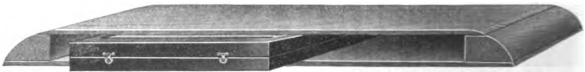
Fig. 678.—The author's "plate tunnel." Strong enough to sustain the patient's weight, but transparent to the x-ray. So large that the plate, in its holder with or without an intensifying screen, may be positioned without moving the patient.
