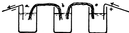
Fig. 187.—Series of electrolytic cells connected by moistened strands of asbestos. Products liberated at extremities only.
