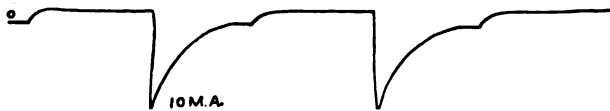
Fig. 311.—Character of faradic current from a long secondary coil with an iron core.
