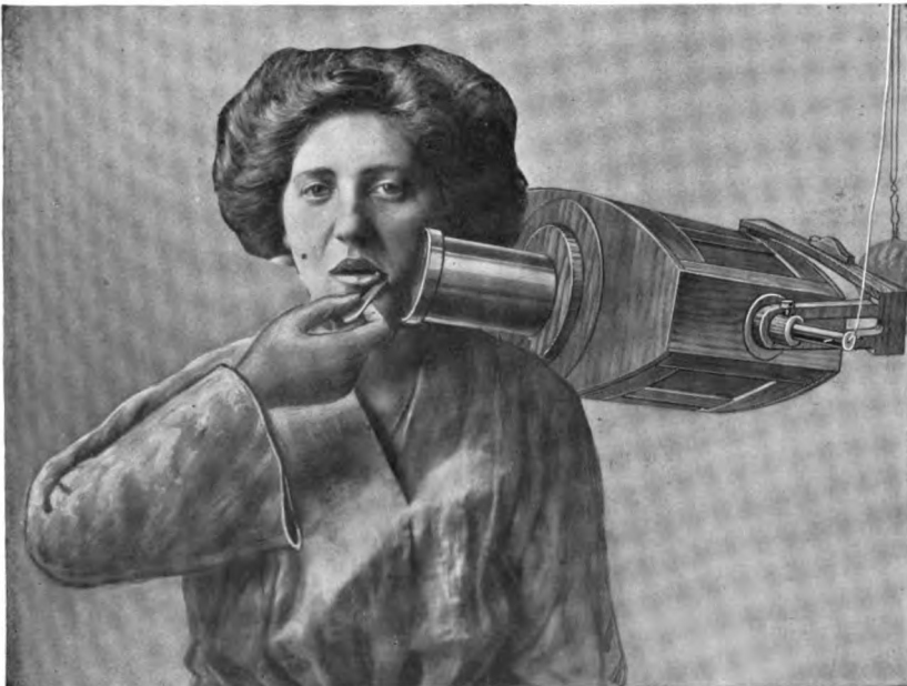
Fig. 579.—Use of the author's vertical film-carrier. Ripperger shield with disk of sole leather in orifice as a protective screen for soft rays.
