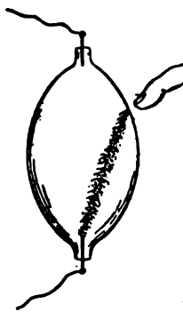
Fig. 389.—Geissler tube, showing cathode stream.
