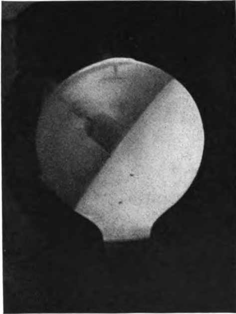
Fig. 512.—X-ray tube showing proper "line" of demarcation between the illuminated and the dark hemispheres.
