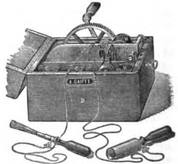
Fig. 90.—Magneto-electric machine for therapeutic use.
