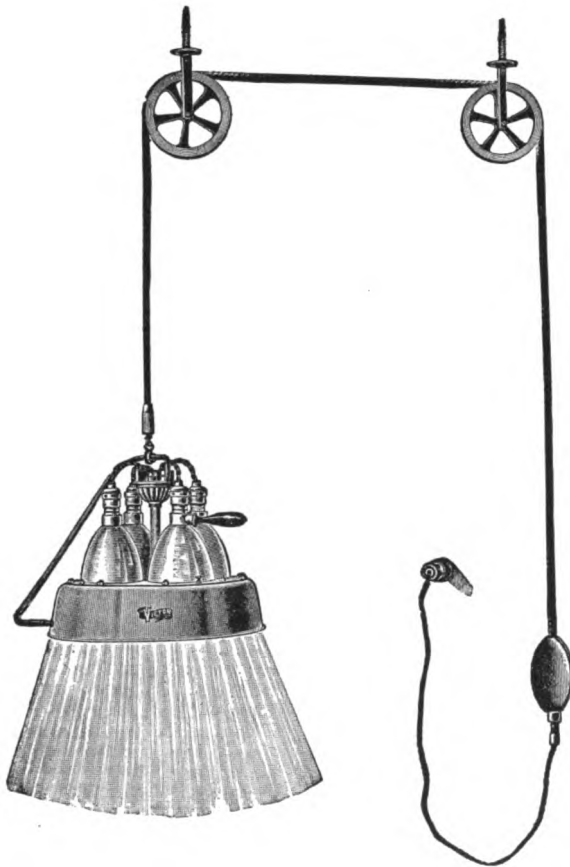
Fig. 403.—Therapeutic lamp with four 125-candle-power incandescent bulbs.
