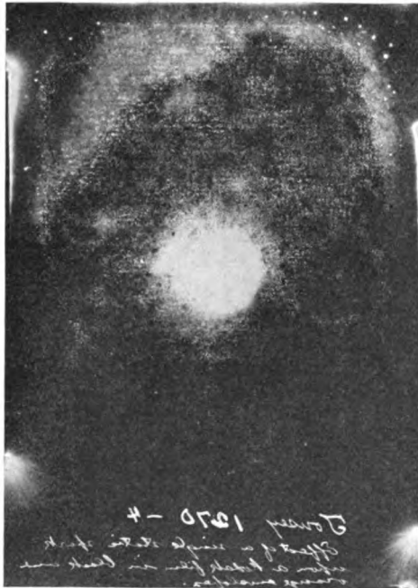
Fig. 38.—Effects of disruptive and convective discharge upon a photographic film in light-proof envelopes.
