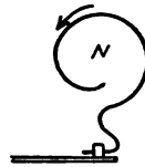
Fig. 82.—Magnetic polarity induced by current in the direction of a left-hand spiral.
