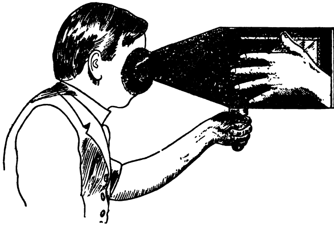
Fig. 445.—The Johnston fluoroscope. The operator stands at one side instead of in a direct line with the rays.
