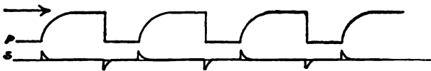
Fig. 115.—Currents in an induction coil with a long secondary wire and no iron core: P, Primary; S, secondary.
