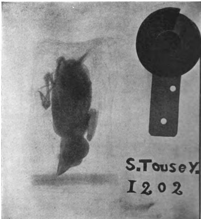
Fig. 520.—Radiograph of young sparrow. Benoist's radiochromometer showing rays No. 3.
