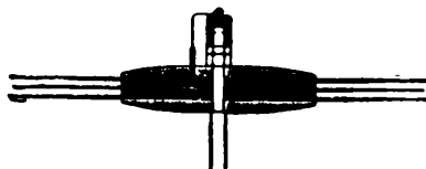
FIG. 19.—Arrangement for electrifying a third or middle steel disk to sparking potential while spinning.
