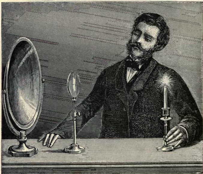
FIG. 167.—IMAGE BY CONCAVE MIRROR.
